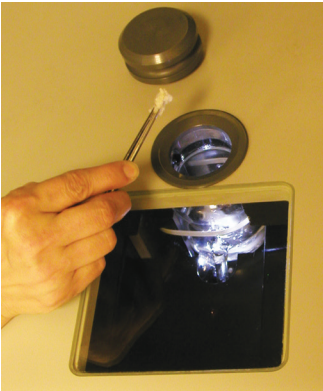
Sample cups of fiber snippets for individual animal fiber diameter testing by Sirolan LaserScan instrument.
